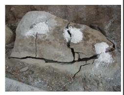
Sylentmite can be used alone or in conjunction with traditional demolition methods to help cut costs, work time and increase safety.
